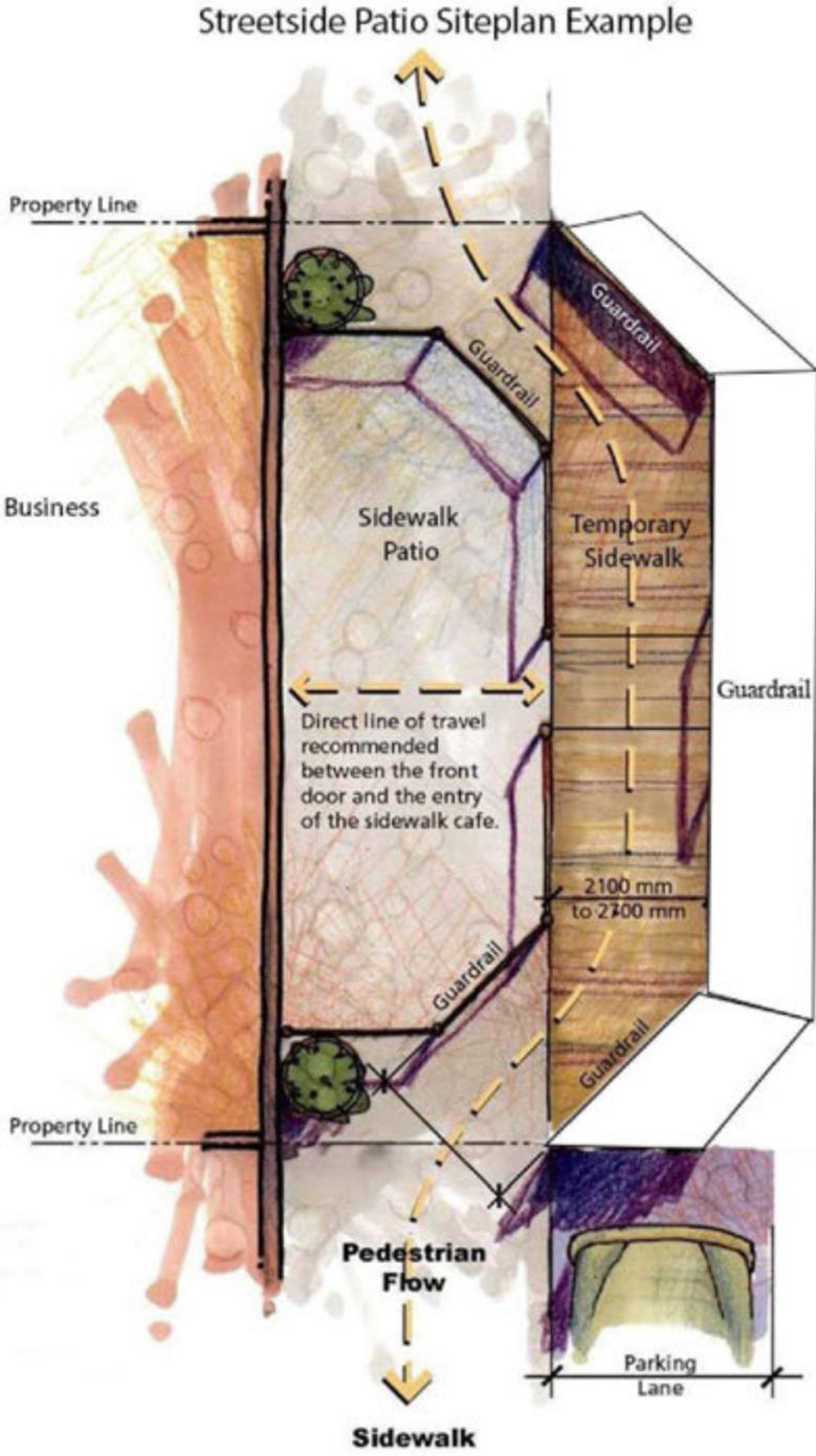
Siteplan should include a list of the types of construction materials used, and the height of objects. Siteplan should also include any infrastructure such as trees, utility poles, etc.
